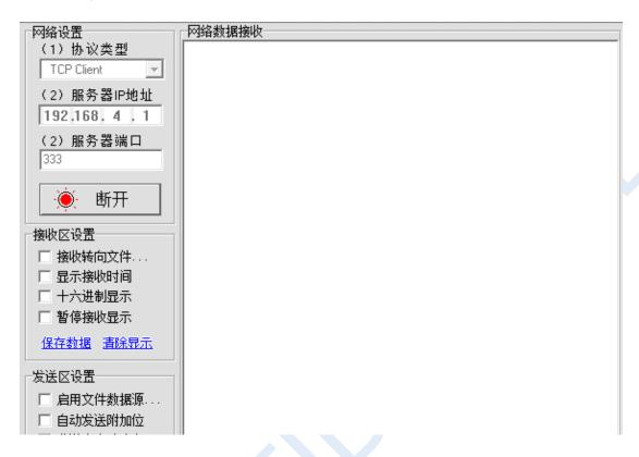
Note: ESP8266EX acting as server has a timeout mechanism. When connection is established and no data is transmitted within a period of time, it will disconnect the client. Please setup a recurring packet transmission every 2s on the computer to ensure connection is maintained.
